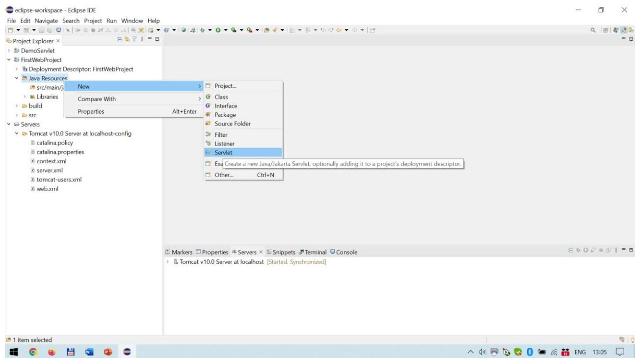
Set servlet name and package in dialog **Create Servlet**, and do not change other parameters when moving to the next steps.
